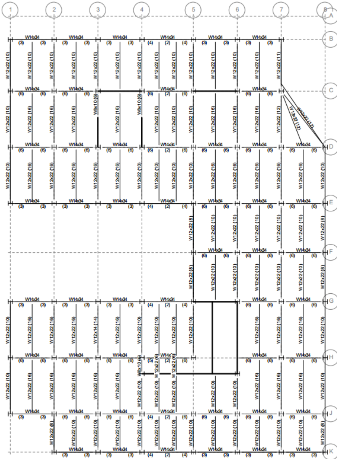
Figure 25: Typical Apartment Framing
