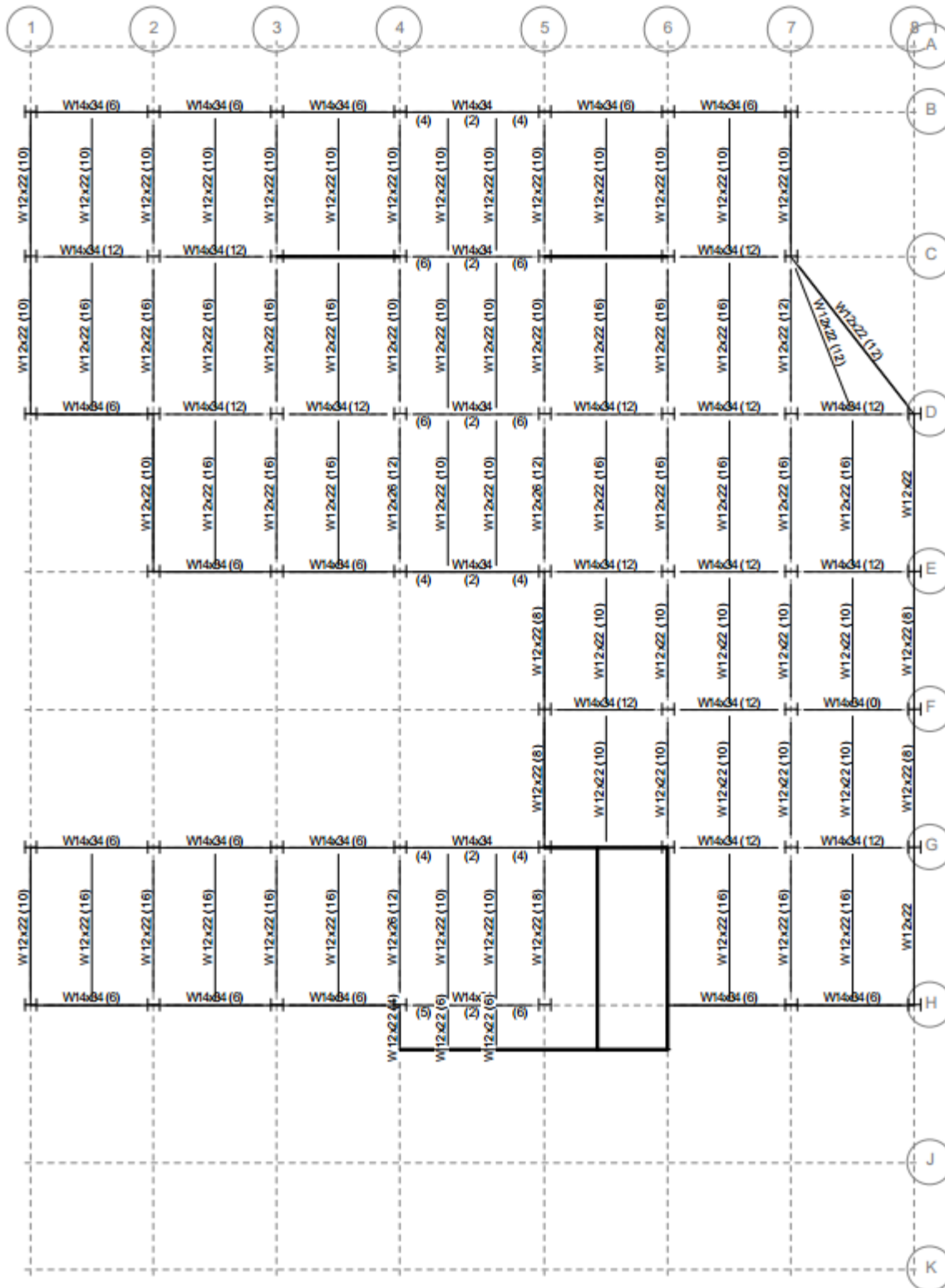
Figure 26: 16 th Floor Framing
